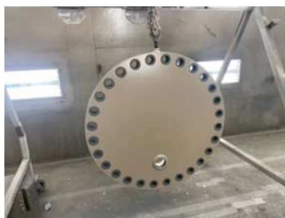
Fabricated 30-inch blind flange before (left) and after (right) coating application for the Second Lower Feeder shutdown
