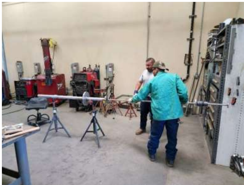
Staff fabricating new injection lance for the fluoride system at the Weymouth plant
