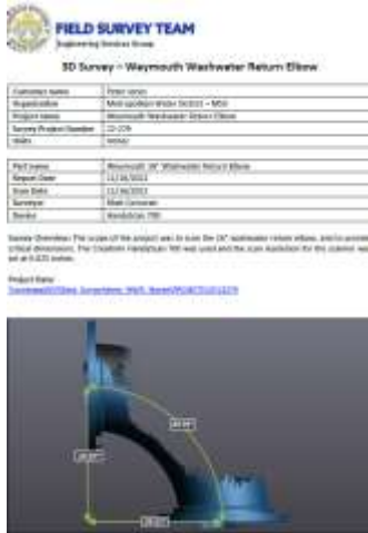
Survey report of the existing elbow (left), fabrication of new elbow (middle), and installed new elbow (right) at the Weymouth plant
