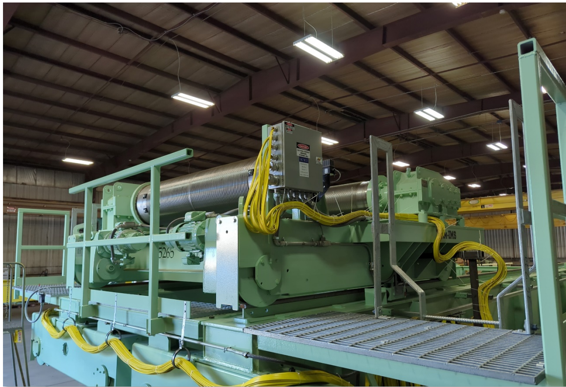
Newly fabricated overhead crane for Iron Mountain Pumping Plant
