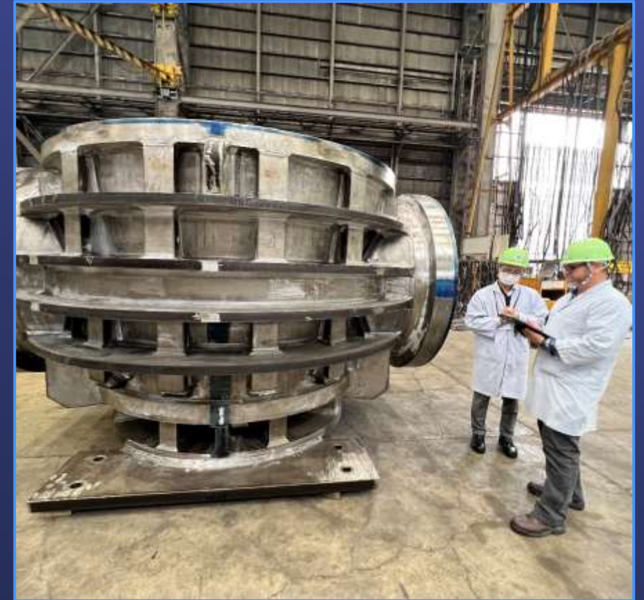
54-inch Diameter Valve Inspection (Japan)
