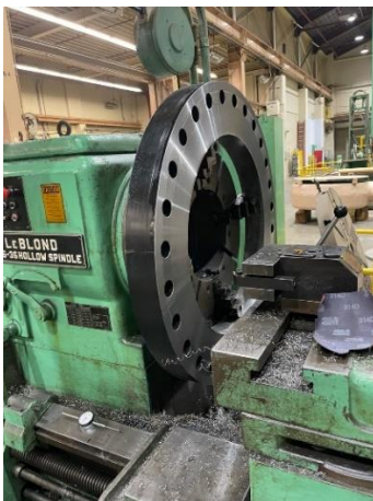
Machining of 28" flange (left), and welding of downstream (center) and upstream (right) spools at the La Verne Shops
