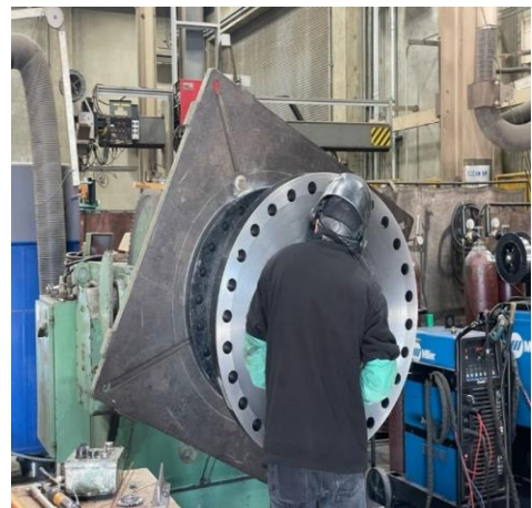
Machining of 28" flange (left), and welding of downstream (center) and upstream (right) spools at the La Verne Shops
