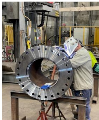
Machining of 28" flange (left), and welding of downstream (center) and upstream (right) spools at the La Verne Shops
