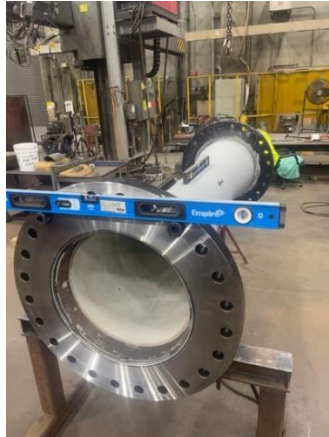
Masking for initial blast (left), fitting of flanges to meter (center) and completed welding of flanges to meter (right) at the La Verne Shops
