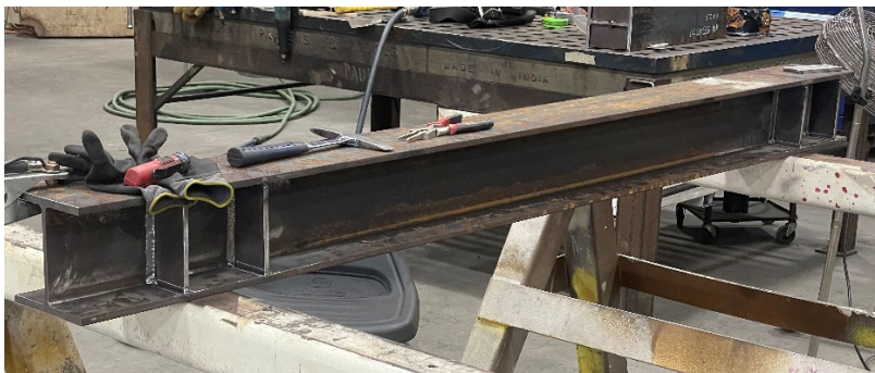
Structural cross-member being fabricated (left) and completed main beam (right) for the AMP bypass line at OC-88
