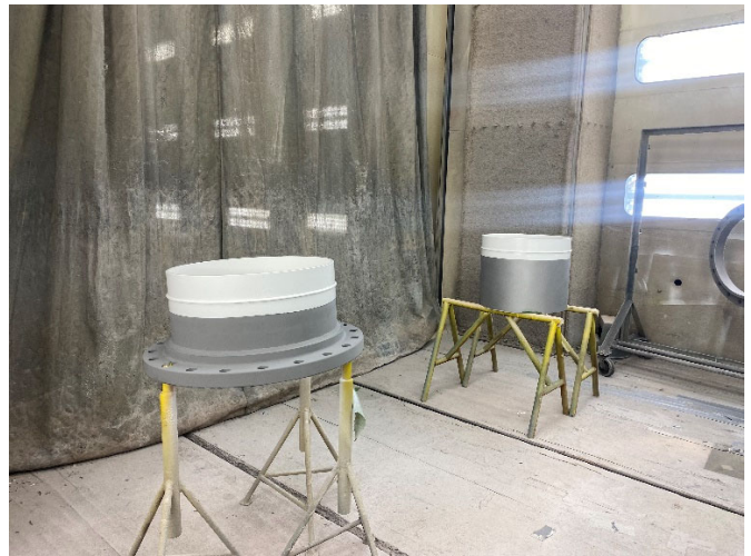
La Verne Shops completed 24-inch compound elbows (left) and thimbles (right) for the AMP bypass line at OC-88
