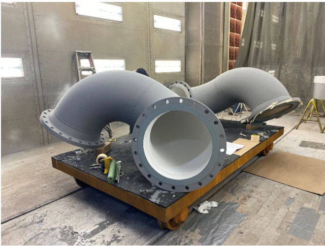
La Verne Shops completed 24-inch compound elbows (left) and thimbles (right) for the AMP bypass line at OC-88
