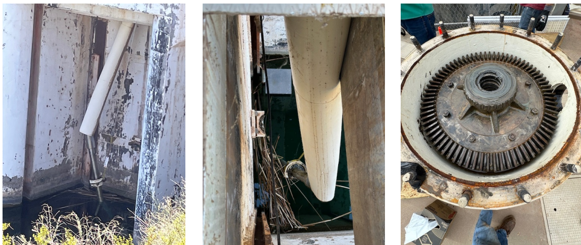
Damaged gate shaft (left and center) and as-found actuator assembly (right) for the gate at Copper Basin
