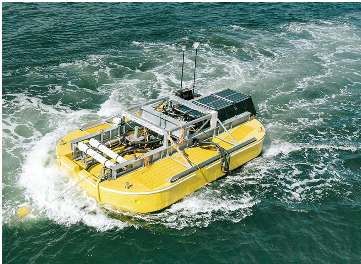
Figure 3.4 Wave Powered Offshore Desalination Facility (Courtesy of Oneka)
