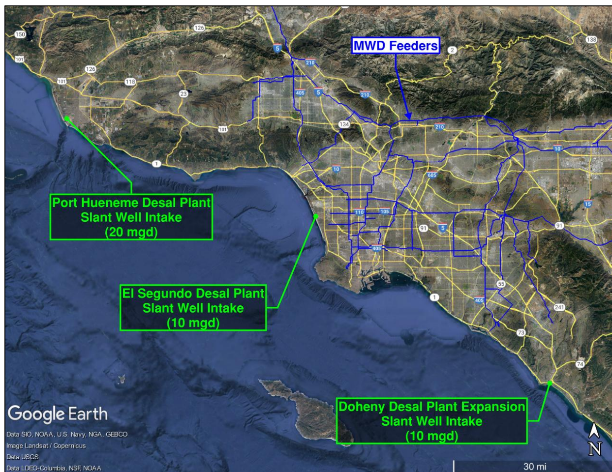
Figure 5.3 Map of Potential Seawater Desalination Facilities
