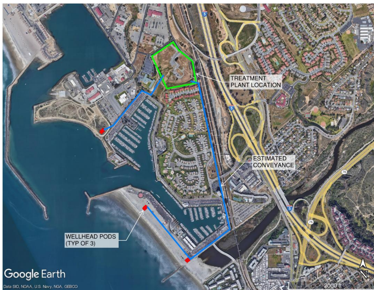
Figure 4.3 Potential Oceanside Seawater Desalination Plant Location
