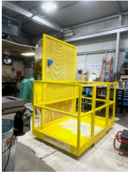
Rebuilt forklift aerial work platform
