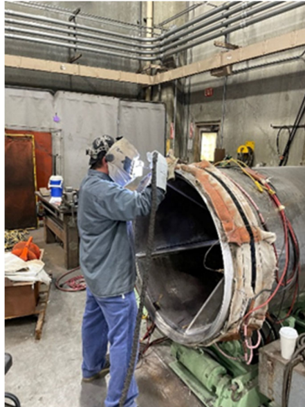
As-found valve gate (left), welding repairs of valve gate (middle) and machining of inner valve body (right)
