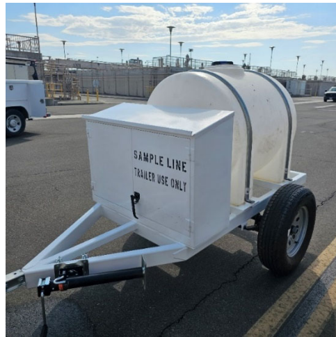
Sample line chlorination trailer refurbished at the Skinner plant
