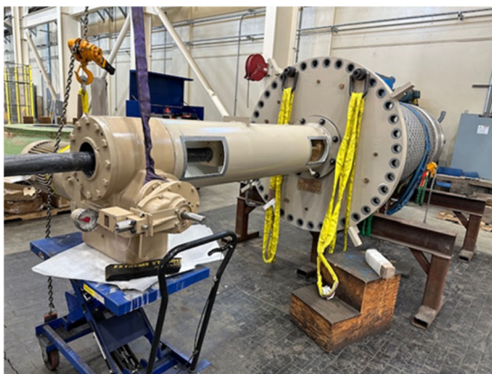
Installation of actuator (left) and completed sleeve valve (right)
