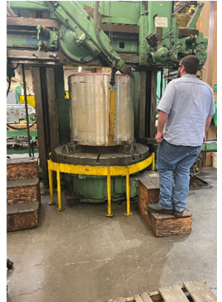
As-found valve gate (left), welding repairs of valve gate (middle) and machining of inner valve body (right)
