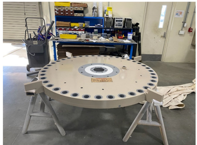
As-found sleeve valve cover (left) and completed valve cover (right)
