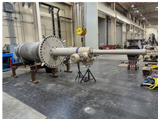
Installation of actuator (left) and completed sleeve valve (right)
