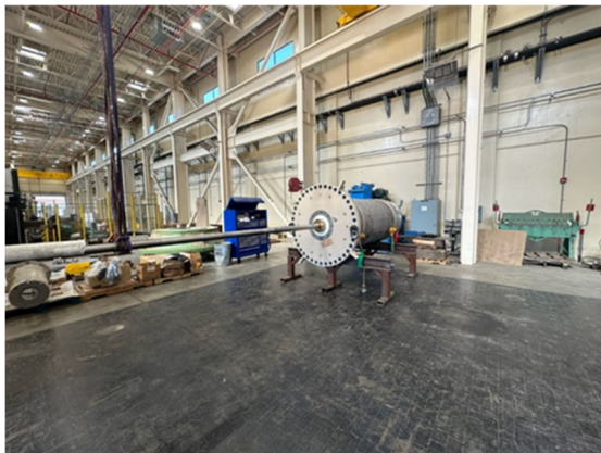
Machining of new lower valve body (left) and assembly of sleeve valve components (middle and right)
