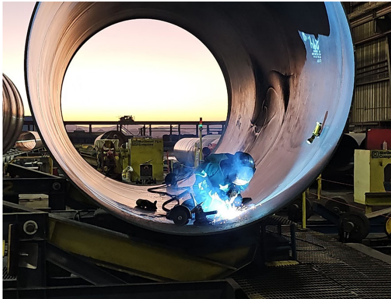
Fabrication of Steel Liner for Lakeview Pipeline
