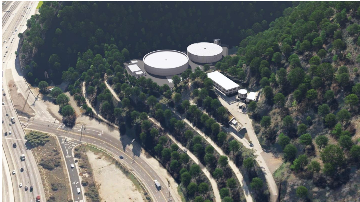
Rendering of the future Sepulveda Feeder Pump Station at the Sepulveda Canyon Pressure Control Facility
