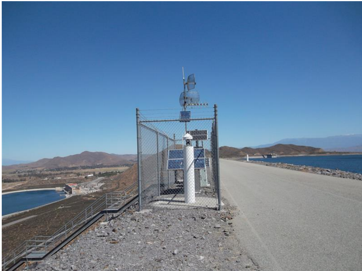
Existing remote monitoring unit and seismic accelerograph in the west crest of DVL dam
