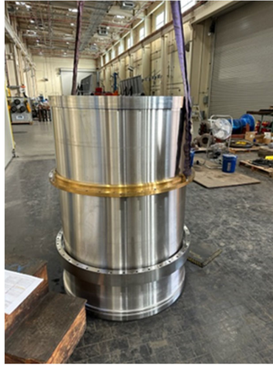
Machining of new lower valve body (left) and assembly of sleeve valve components (middle and right)
