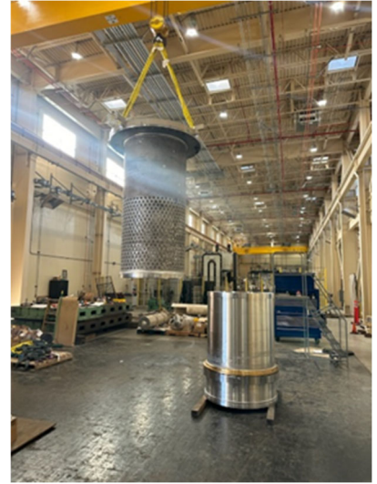
Machining of new lower valve body (left) and assembly of sleeve valve components (middle and right)
