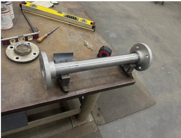
Damaged equipment, fabricating new stainless-steel stub shafts & replacement of equipment
