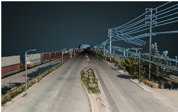
Colorized point-cloud: looking northerly along Alameda Street. The clearly visible overhead wires are a key benefit provided by the technology.
