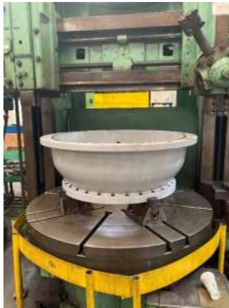
Conducting as-found dimensional check of blasted siphon breaker body for DWR's Dos Amigos Pumping Plant
