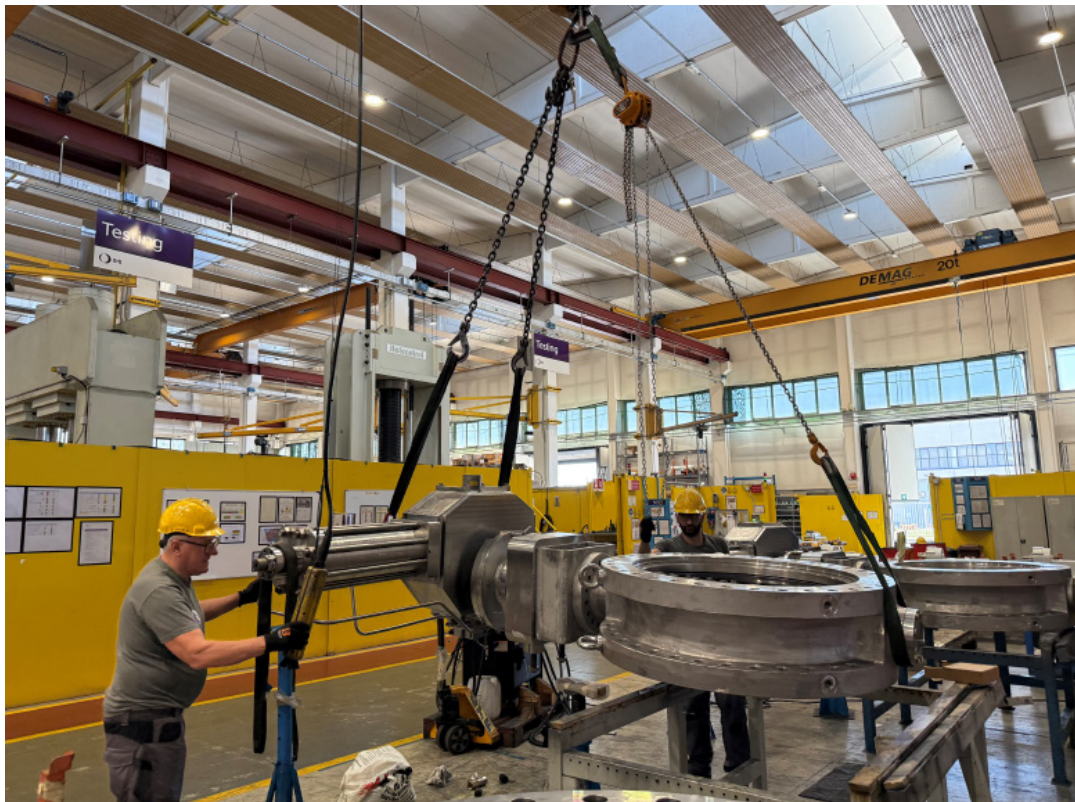
Lake Skinner Tower Valve Procurement Performance Testing of 42-Inch Butterfly Valves
