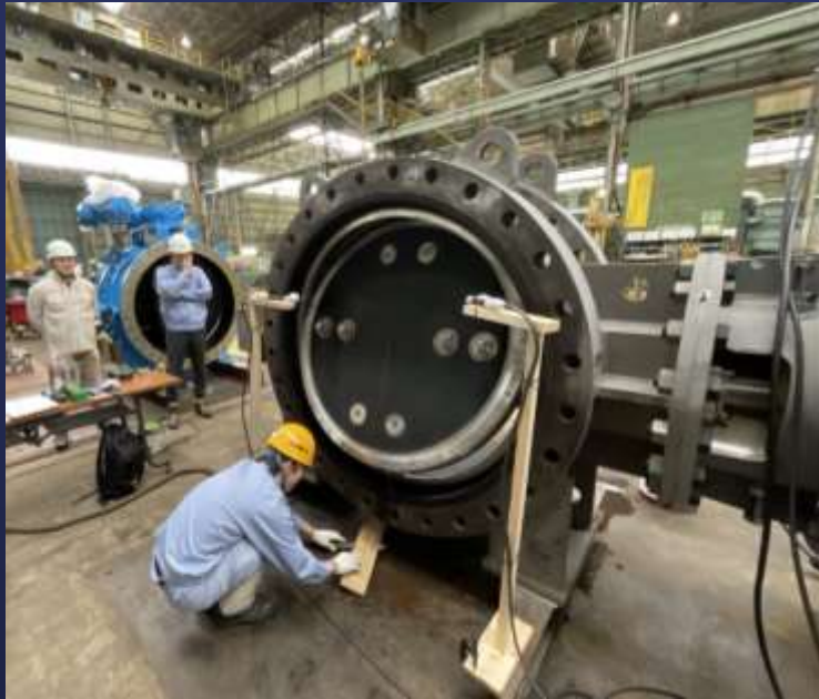
Foothill Pump Station – Inland Feeder Intertie Butterfly Valve Fabrication
