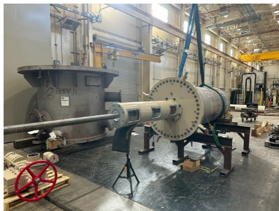
Repaired valve gate and new stem (left) and refurbished operator pedestal (right) for Auld Valley Control Structure on San Diego Pipeline No. 3
