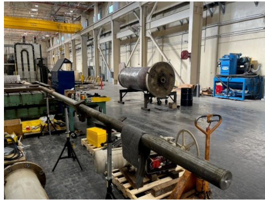
Troubleshooting of Auld Valley Control Structure valve operator (left) and shaft (right)
