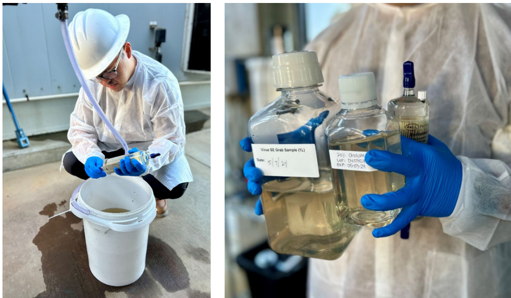
Staff collects samples to evaluate performance of the MBR-based treatment train at the NIC Demonstration Plant
