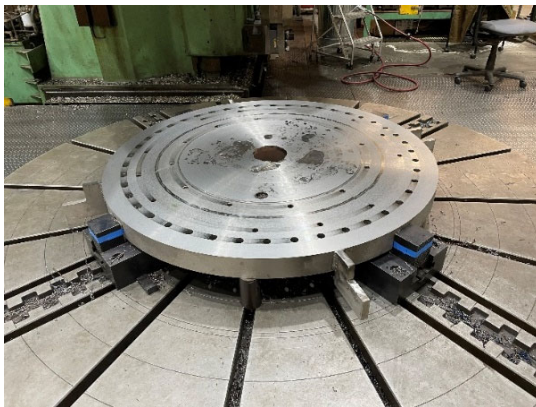
Machining of existing valve cover (left) and manufacturing new bronze stem bearing (right)
