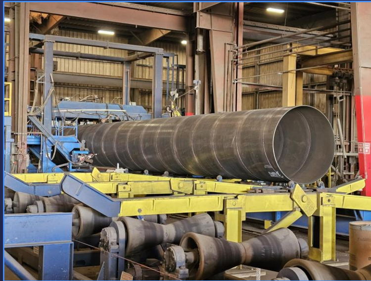
Fabricating Liner Pipe
