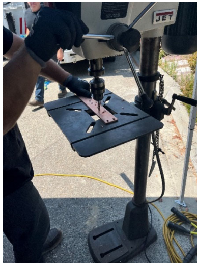
Drilling buss bar for bolting
