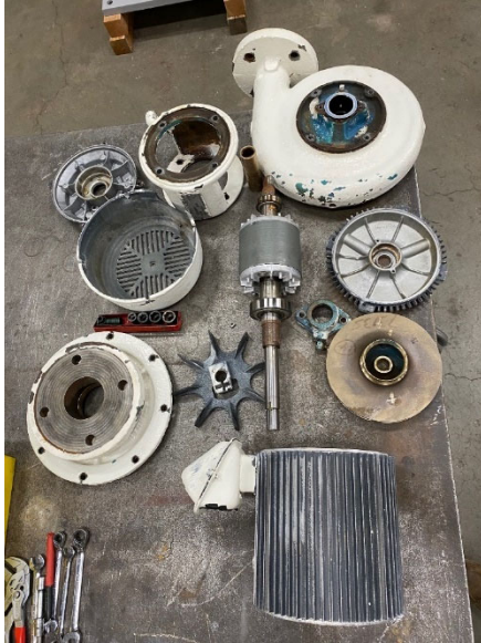
230kV transformer oil pump disassembled and ready for rebuild
