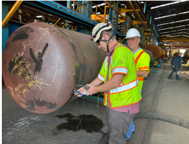
Staff inspecting the inner vessel thickness of a chemical tank
