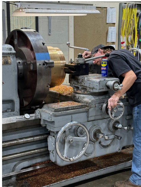
Staff machining a discharge valve component at the Gene pumping plant
