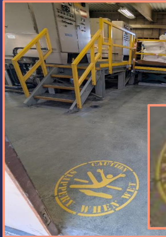
Mills - SRR ( 134 ) Dry Poly spills create slipping hazard Anti-Skid Coating & Stencil Awareness
