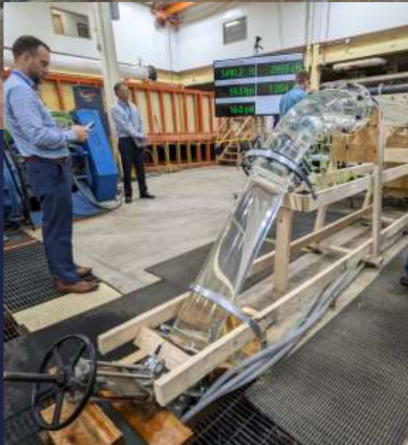
1/32 nd Scale Outlet Works Cavitation Model
