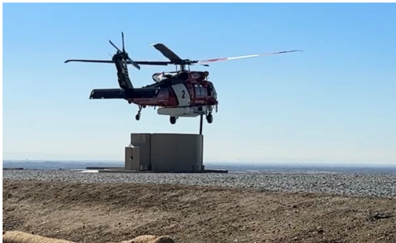
Orange County Fire Authority testing the new Heli-Hydrant at the Diemer plant
