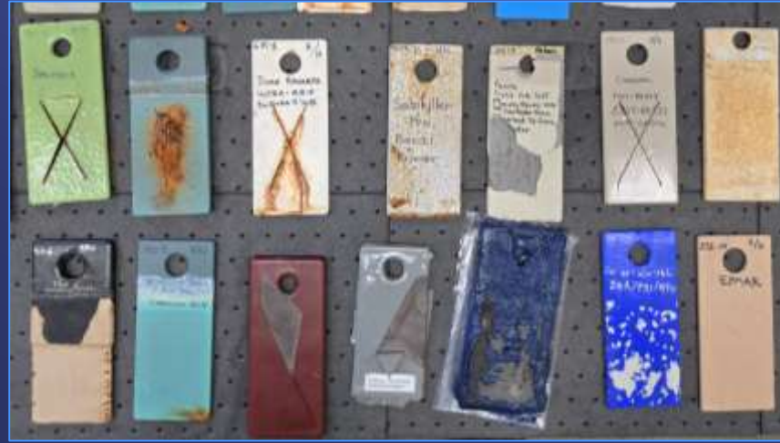
Failed Coating Test Coupons
