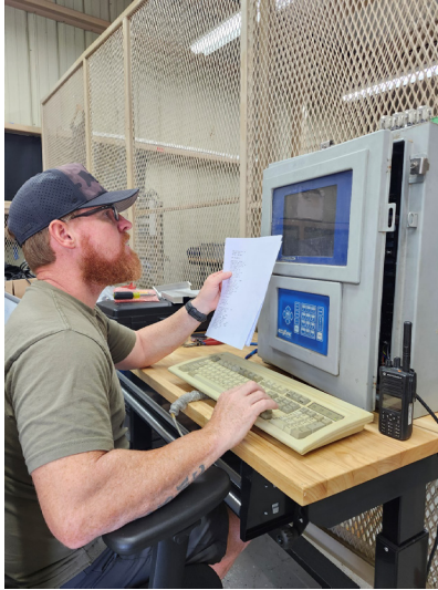
Staff configuring flowmeter parameters after repair
