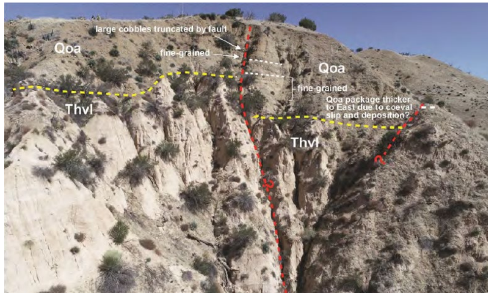
Figure 8-3: Drone Image of San Gabriel Fault (Palomas Segment) fault strand displacing base of Older Alluvium (Qoa) deposit (yellow dashed line)
