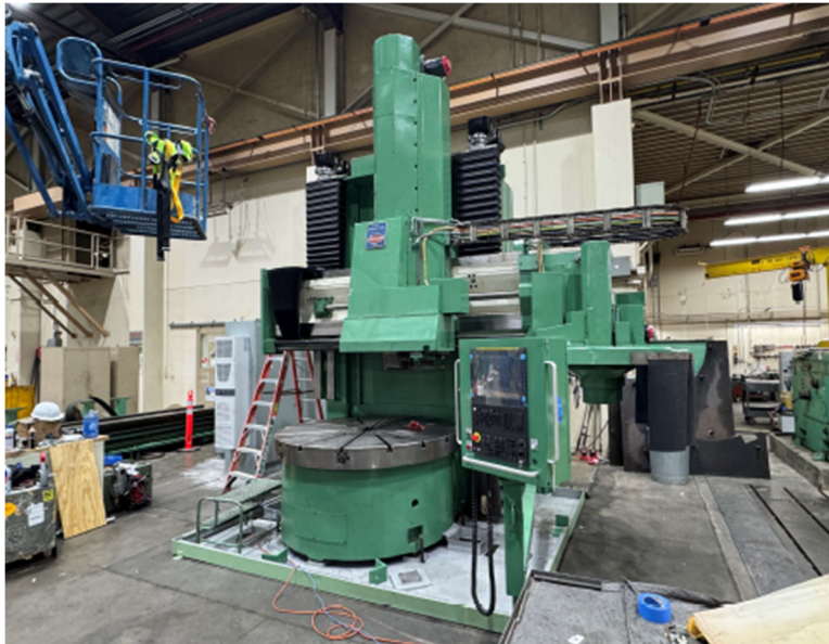
La Verne Shops Improvements — Installing New Bellows for Refurbished Vertical Turning Lathe
