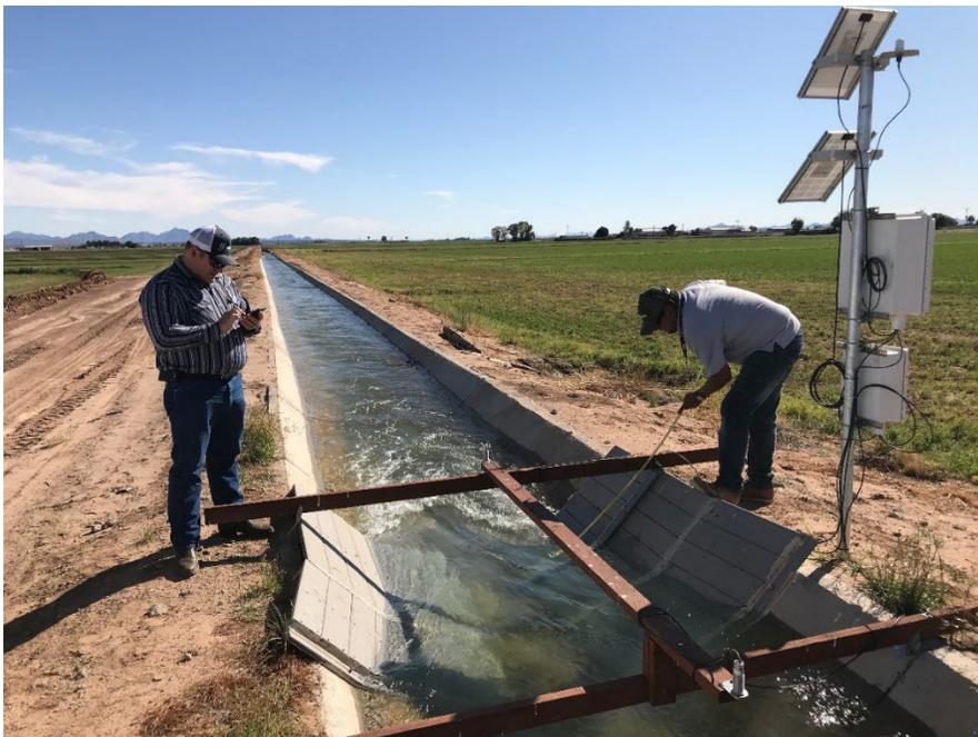
Figure 7. A flume used to measure irrigation flows on Metropolitan farmland in 2017. (photo by Metropolitan)
