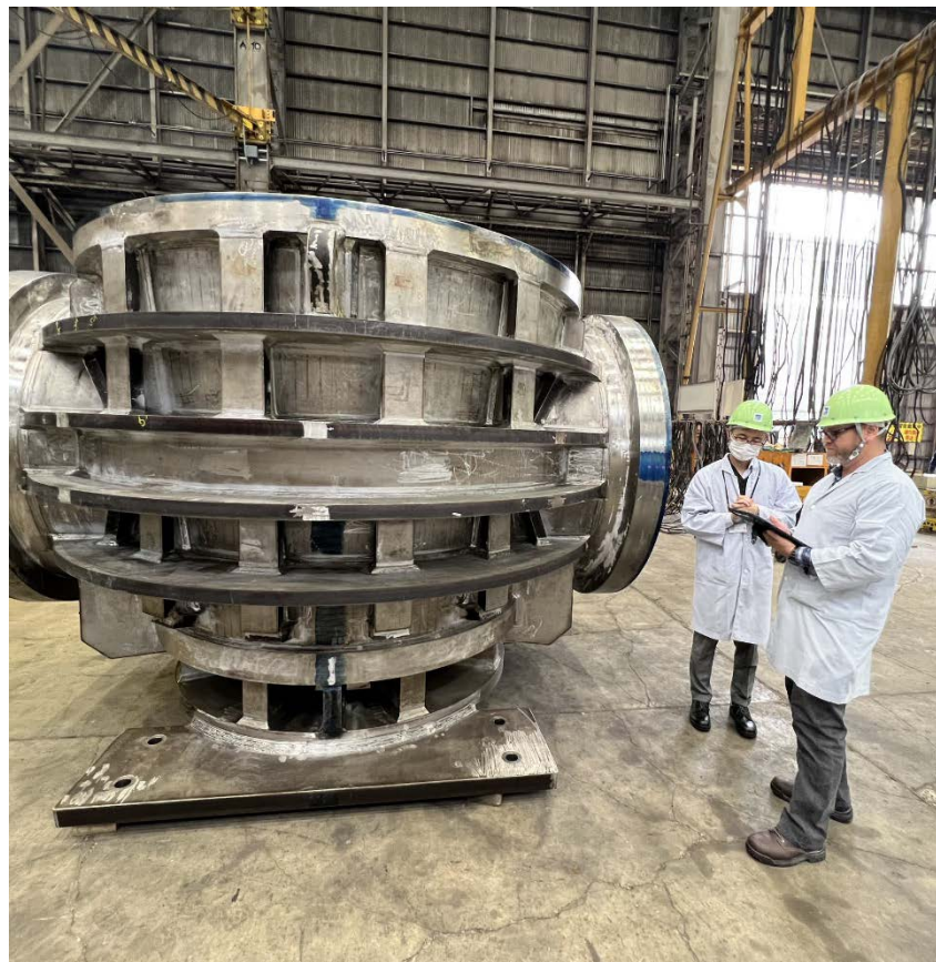
Third-party inspector and Metropolitan construction inspector performing inspection of 54-inch diameter valve
