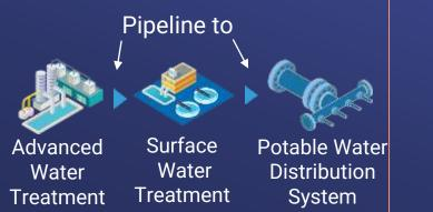
Direct Potable Reuse Raw Water Augmentation
