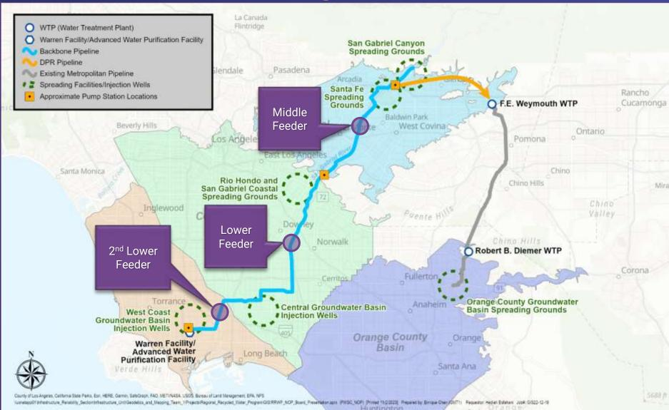
DPR by way of treated water augmentation is the planned introduction of recycled water **directly into** a public water system
