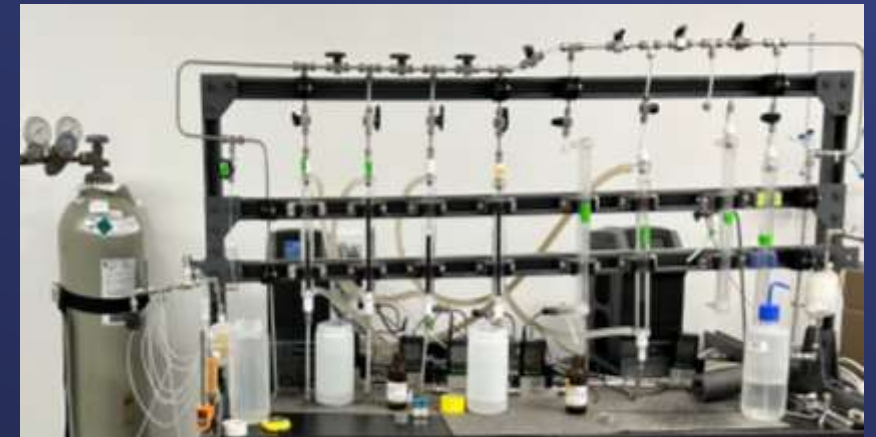
Bench-scale GAC testing setup
