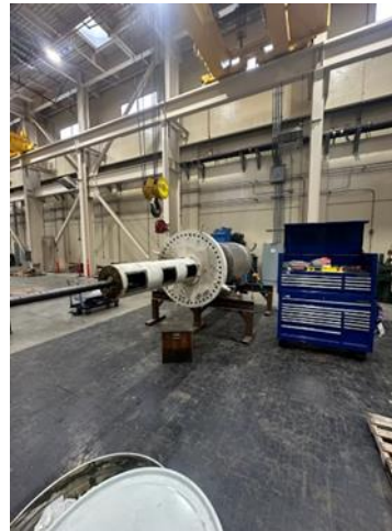
Auld Valley PCS sleeve valve received at La Verne Shops for refurbishment
