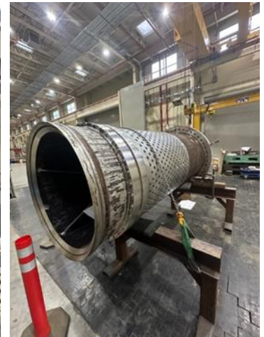
Auld Valley PCS sleeve valve received at La Verne Shops for refurbishment
