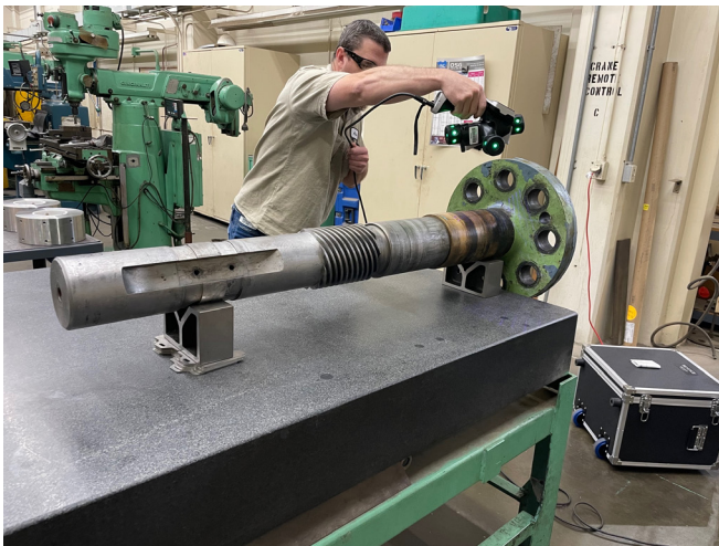
Staff performing dimensional inspection of discharge valve plug shaft (left) and resulting three-dimensional rendering (right)
