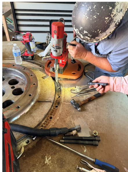
Staff repairing Eagle Unit 1 impeller
