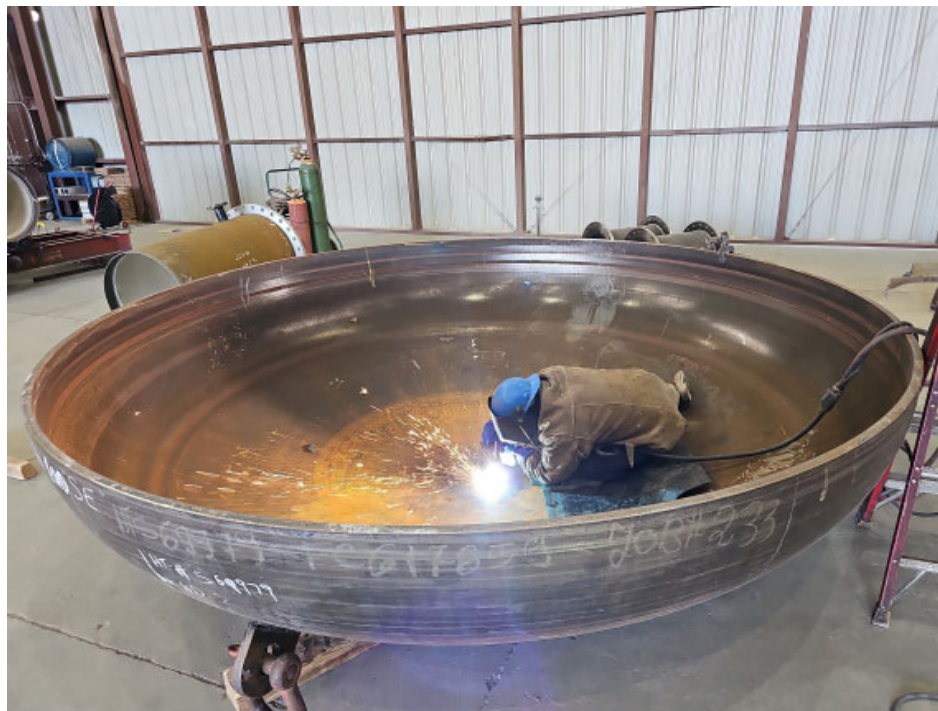
Lakeview Pipeline Procurement – 133.5-inch Bulkhead Fabrication
