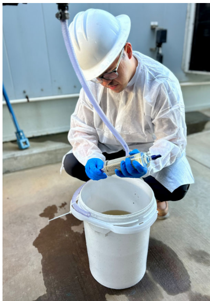
Staff collects samples to evaluate performance of the MBR-based treatment train at the NIC Demonstration Plant
