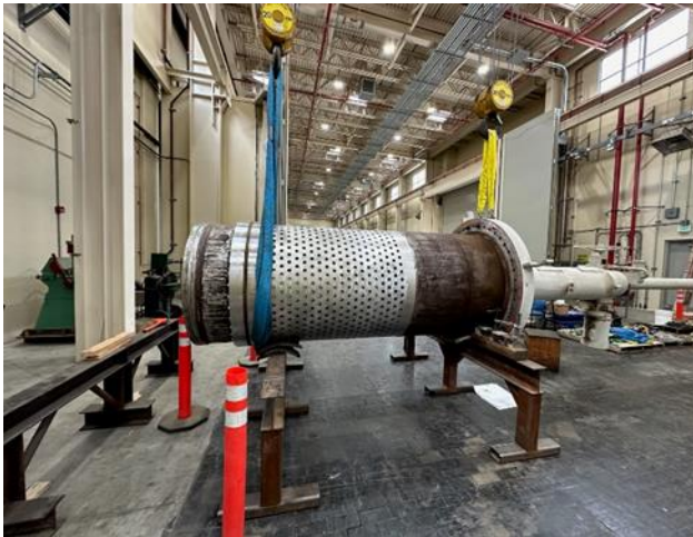
Auld Valley PCS sleeve valve received at La Verne Shops for refurbishment
