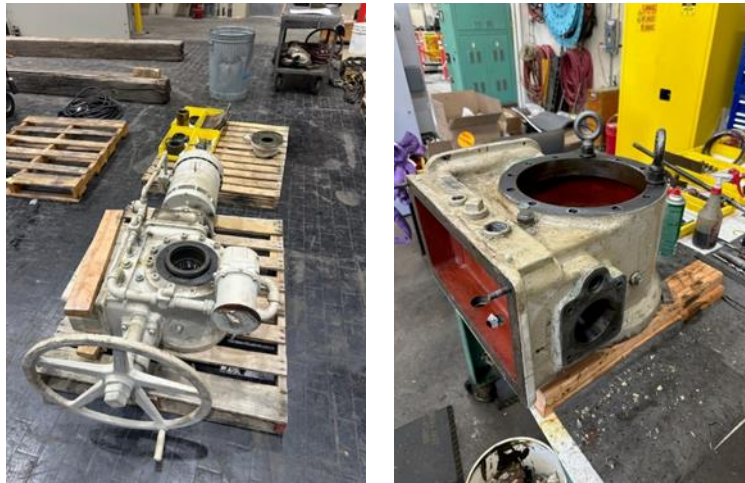
As received actuator (left) and disassembly of actuator (right) at the La Verne Shops for refurbishment
