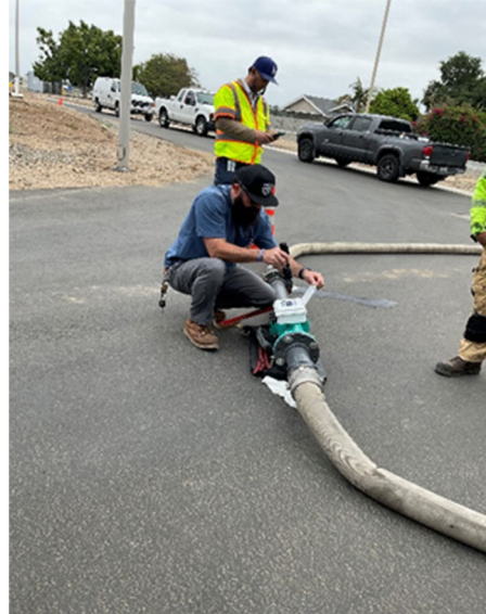
Staff verifying flow rate for the air gap to the sanitary sewer at the Weymouth plant.
