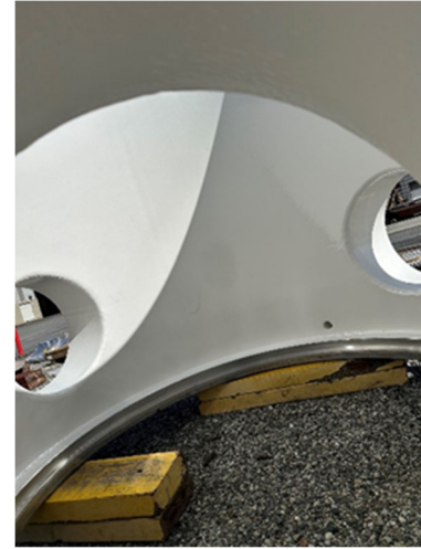
Corrosion on top side (left) and finished coating (middle and right) of a component of the DVL sleeve valve
