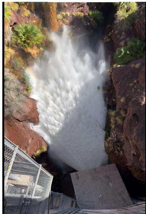
*Fig 2: Captured image of valve open to 60 percent*
