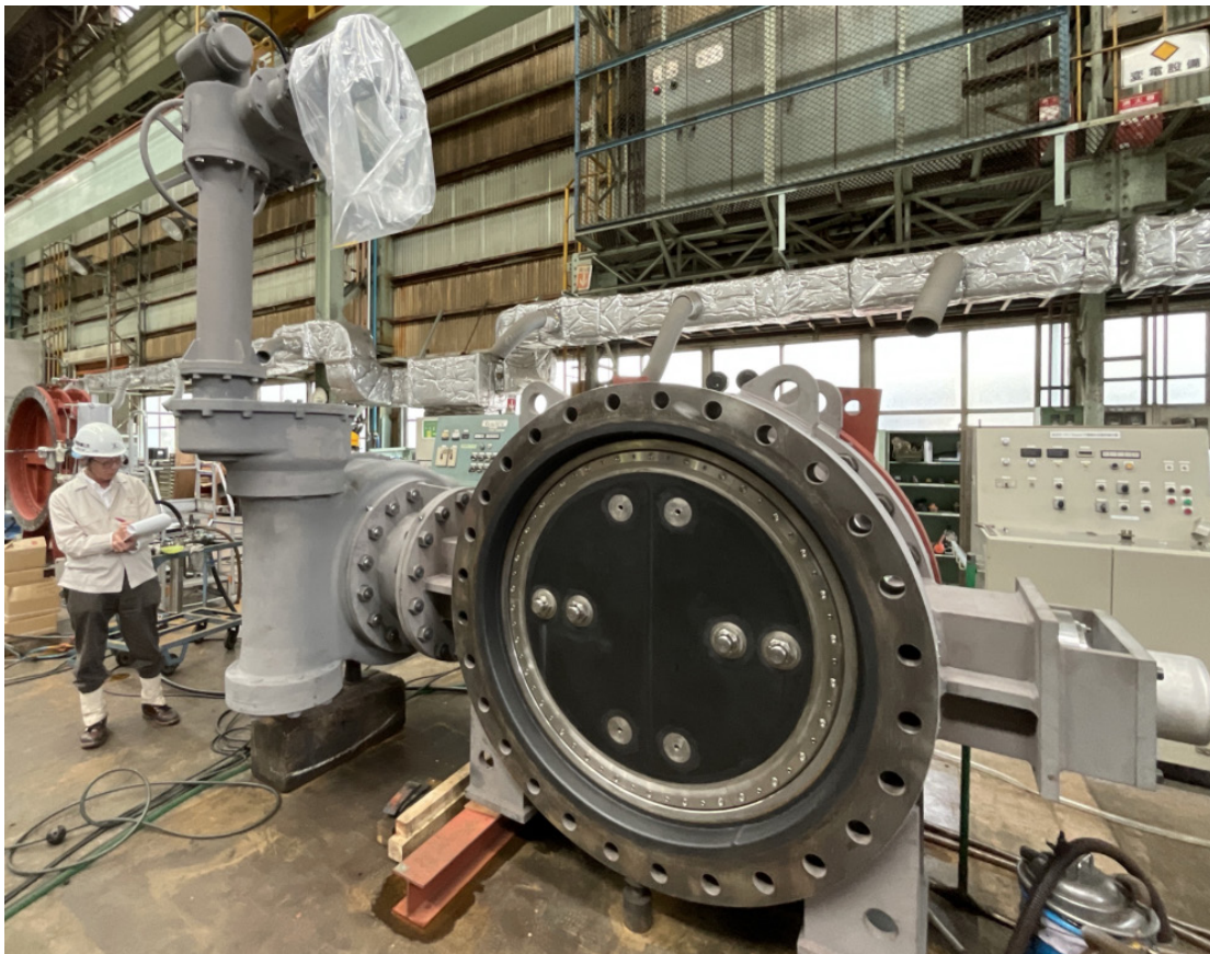
54-Inch Butterfly Valve for Foothill Pump Station Intertie –Butterfly Valve Factory Testing
