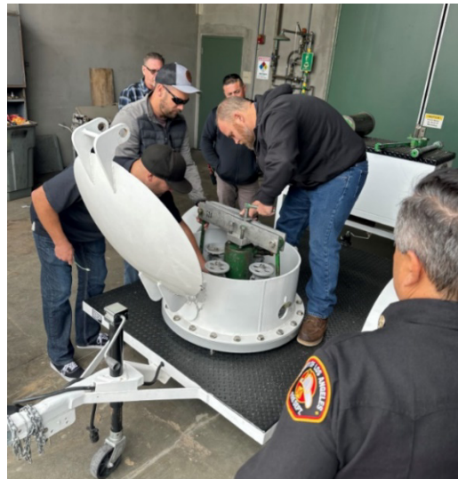
Staff inspecting C-Kit to stop a simulated chlorine leak (left) and installing C-Kit with LACFD observing (right)
