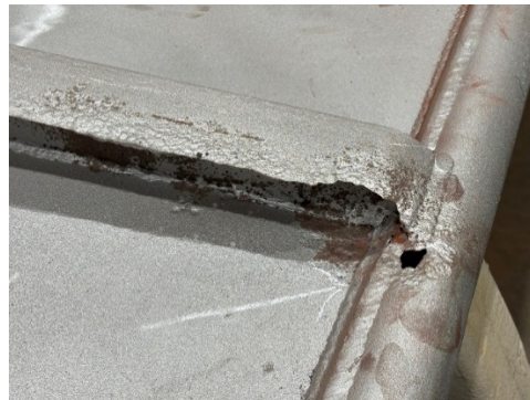
As received condition of wing gates (left) and typical corrosion damage (right)
