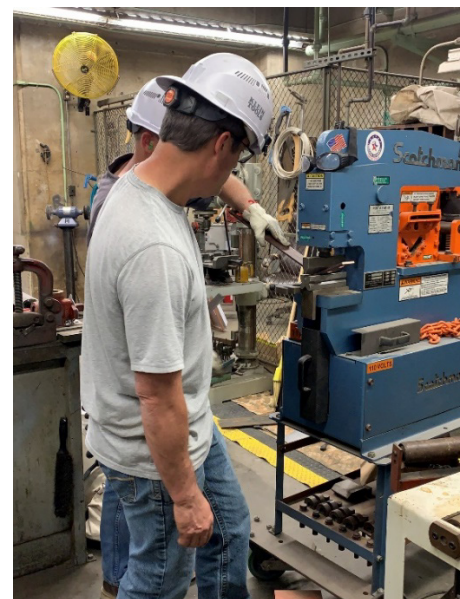
Staff installing spare transformer neutral CT (left) and fabricating bus for neutral CT connection (right) at Hinds pumping plant
