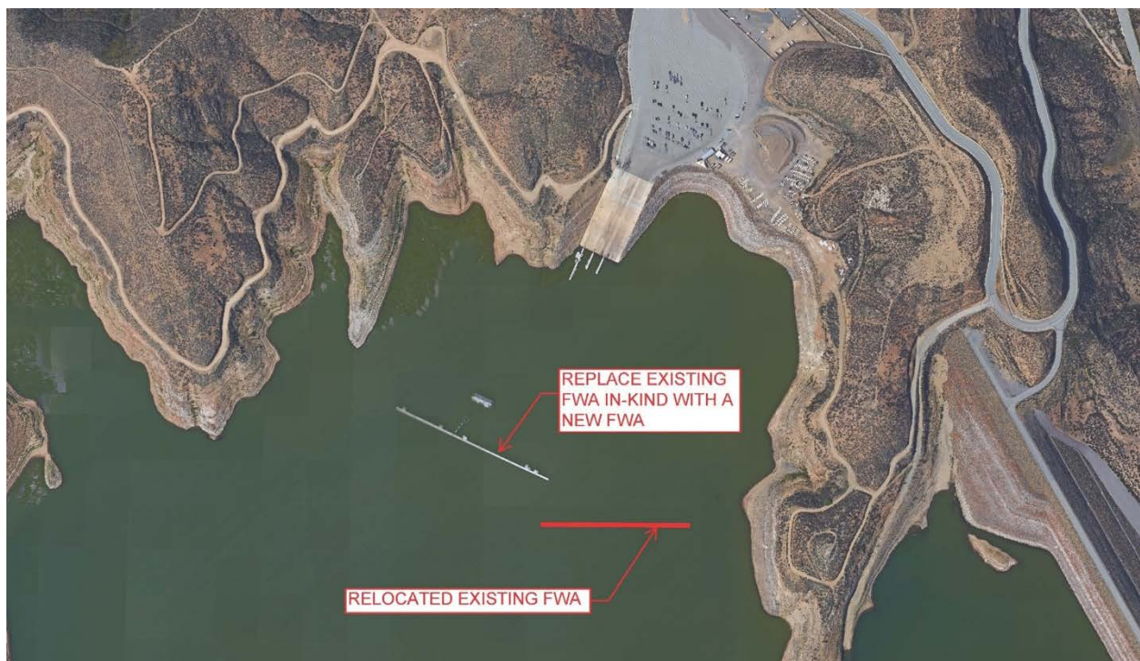
Aerial view of proposed floating wave attenuator (FWA) system at Diamond Valley Lake
