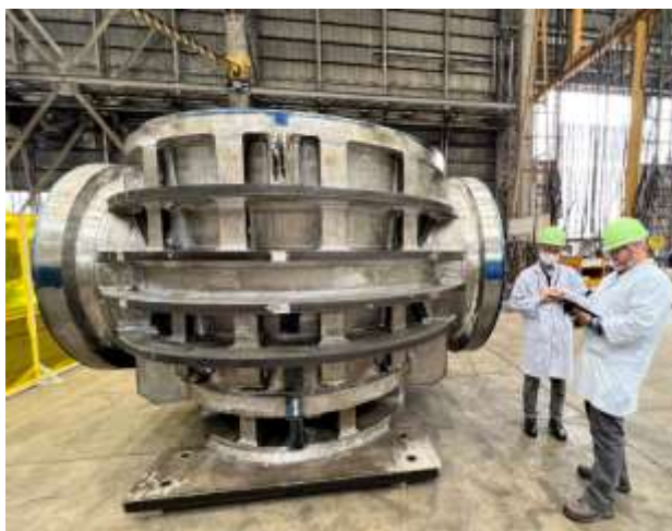
Second Lower Feeder Valve Procurement Conical Plug Valve Body Inspection
