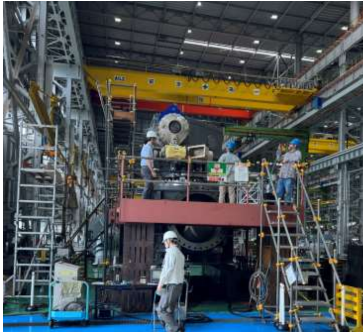
Second Lower Feeder Valve Procurement Conical Plug Valve Shop Performance Testing
