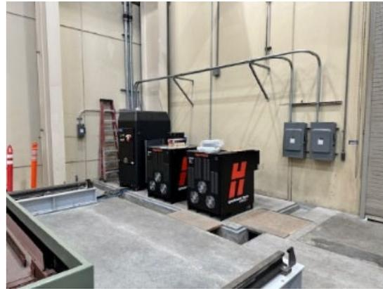
**Partially installed Plasma Arc Cutting System at the La Verne Fabrication Shop**
