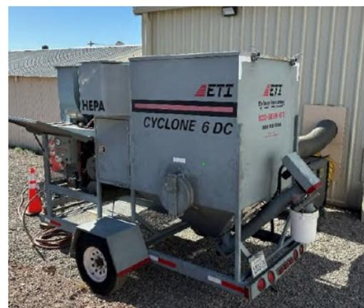
**Abrasive blasting booth and dust collector to be used at Desert facilities**
