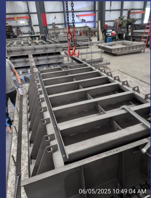
Completed Slide Gates
