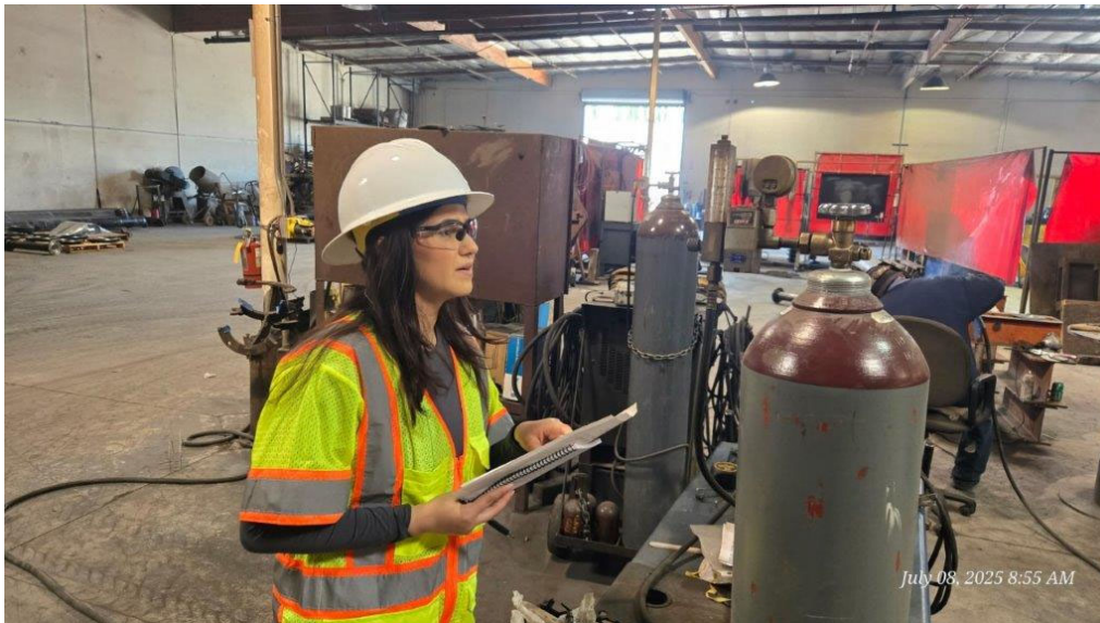
Construction management intern checking the CO2 flow rate on the welding equipment at the La Verne shops
