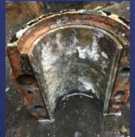
Wear & corrosion on shaft casing
