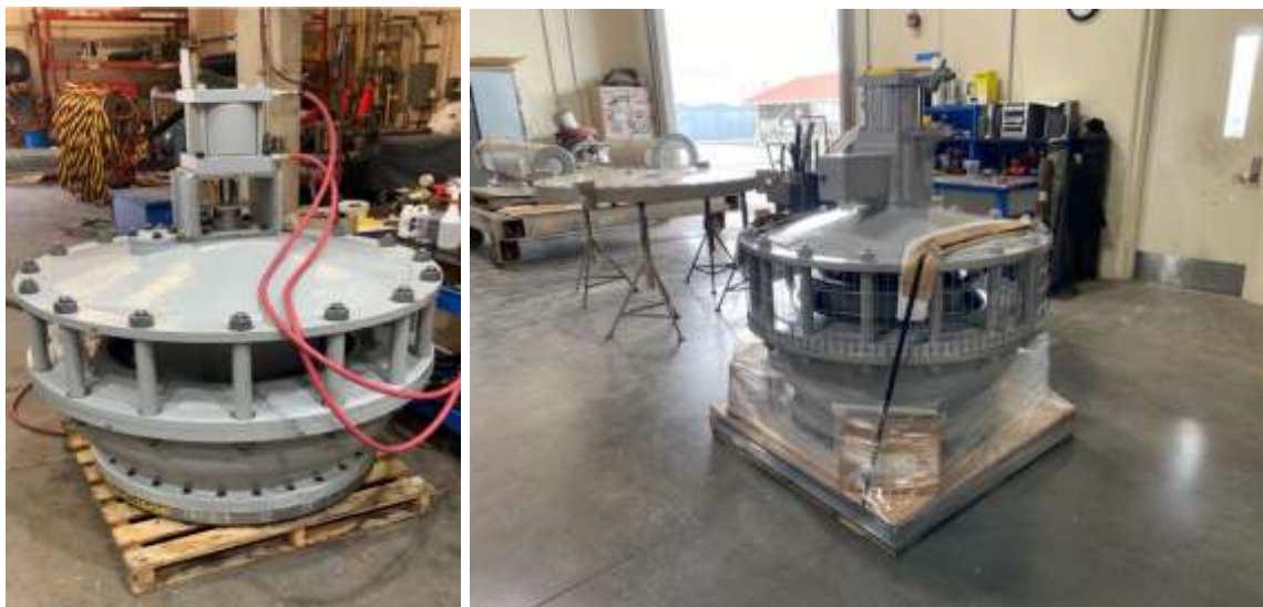
Functional testing of the siphon breaker (left) and completed siphon breaker packaged for delivery (right) from the La Verne Shops to DWR
