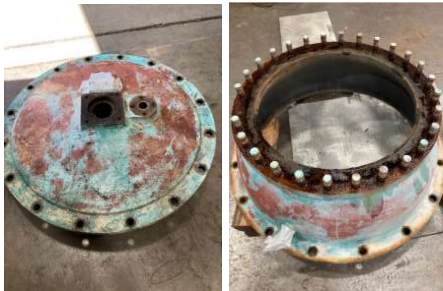
As-received condition of the siphon breaker cover (left) and body (right) for DWR’s Oso Pumping Plant
