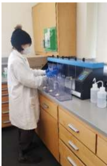
Staff performing jar testing to determine optimal chemical dosage at the Jensen plant
