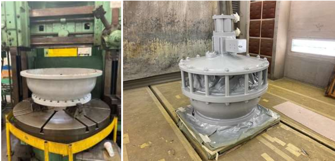
Checking dimensions of the blasted siphon breaker body (left) and final coating of assembled siphon breaker (right) for DWR's Oso Pumping Plant
