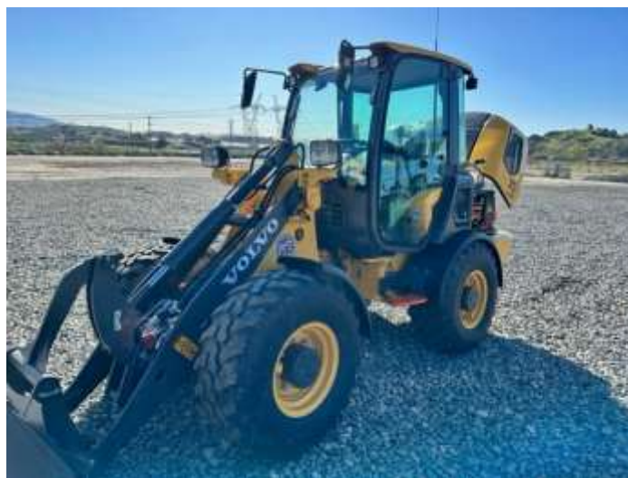
LADWP battery-electric front-end loader at the Jensen plant
