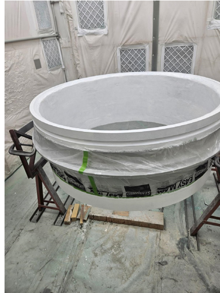
Spool piece prior to repair (left) and spool piece after coating repair (right)
