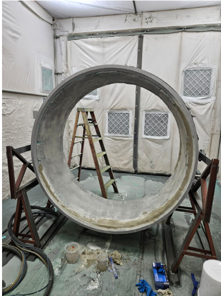
Spool piece prior to repair (left) and spool piece after coating repair (right)
