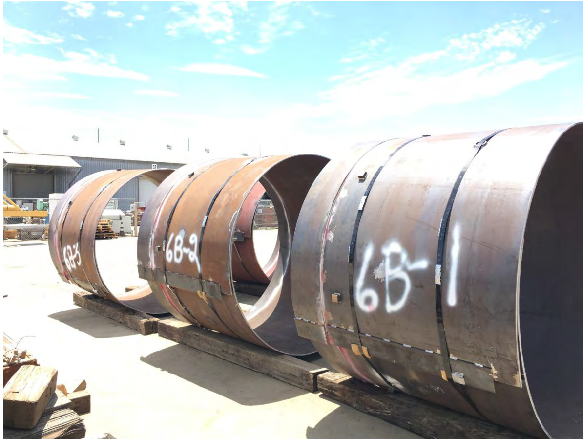
Figure 3. Coiled Steel Pipe Section
