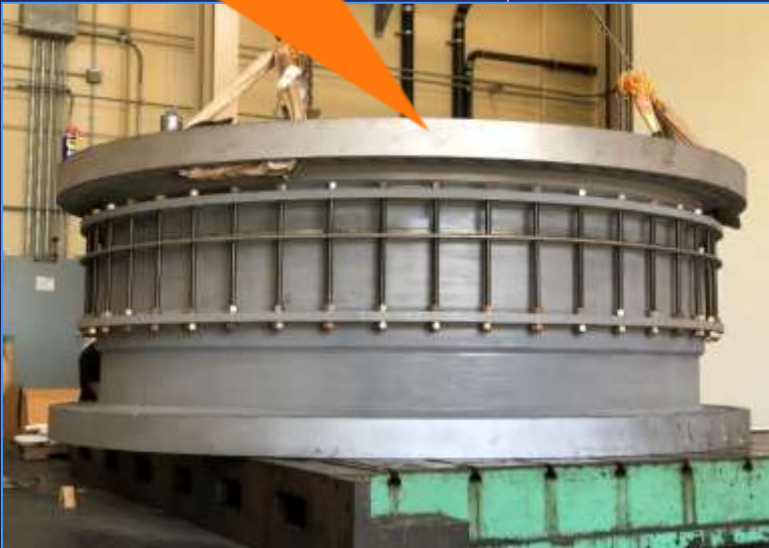
New Slip Joint Completed @ La Verne Shops
