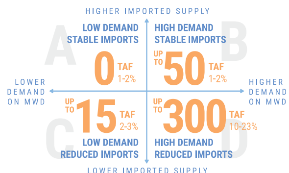
Figure 17: Projected Net Shortage Under Different Supply and Demand Conditions Identified in IRP A, B, C and D Scenarios
