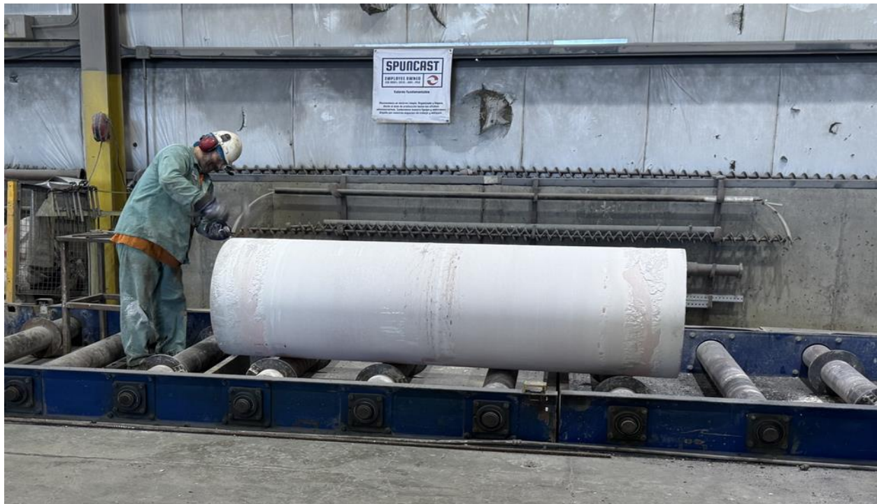
Fabrication of stainless-steel sleeve valve components at the Spuncast facility in Watertown, Wisconsin
