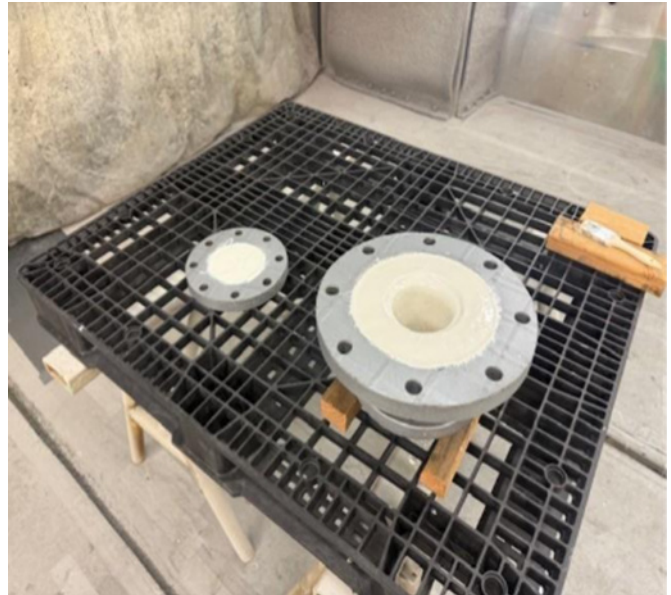
Corroded and patched piping (left) and newly fabricated and coated reducing flange (right) for the Weymouth industrial water system
